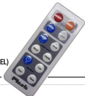
Infrared remote control for adjusting the movement and day light sensor parameters on the light fittings equipped with it. Parameters with which the luminaires are initially delivered are: 100% for the detection area, 50 lx for the daylight level and 1 min. the holding time.
